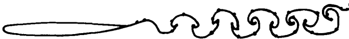
FIGURE 8. Vortex position at tU_\infty/c = 1.85 . 8.4% symmetrical Von Mises aerofoil in pitching oscillation; \nu = 20 , \theta_0 = 0.573^\circ .
